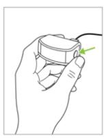
To configure the countdown timer, press and hold the button on the side of the SensorClick motion sensor for 5 seconds until the red LED illuminates. Then press:
