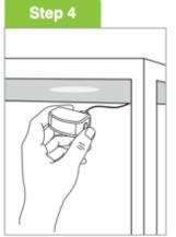
Mount the motion sensor to a flat surface (e.g., under the desk) aiming at the area you wish to detect movement.
