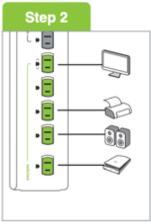
Plug peripheral electronics into the outlets on the power strip labeled "switched".
